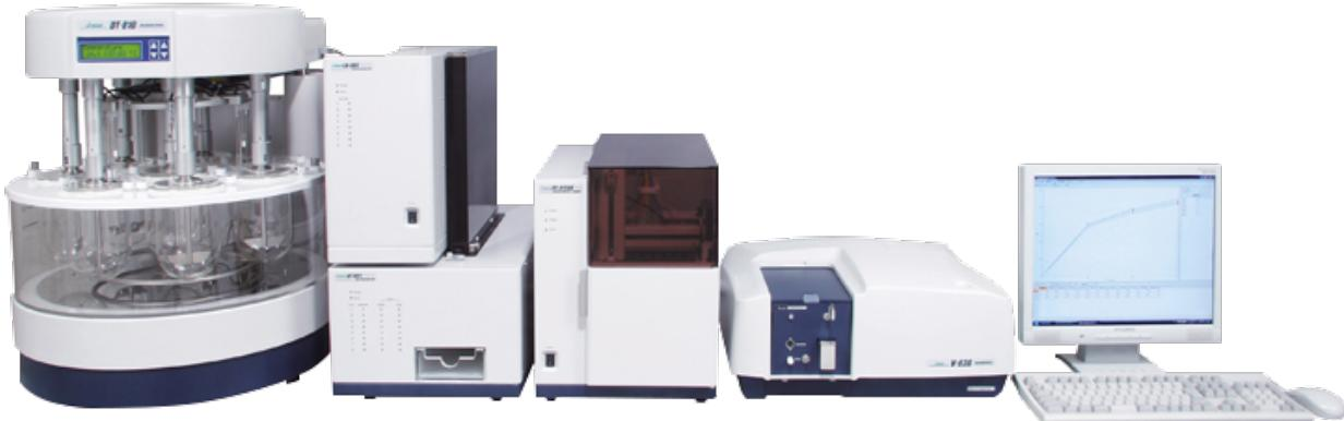
This system includes the LH-SV8 8-position syringe pump and the AF-801 Automated filter changer. It provides automatic filtration of a maximum of 20 ml of sample solutions from all 8 vessels using 25 mm diameter membrane filters with a pore size of 0.45 micron (0.2 micron optional). After each sampling, filters are automatically exchanged. The dedicated software can fully automate the dissolution testing including sample filtering.
