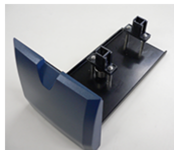
Cuvette height adjustment screw
